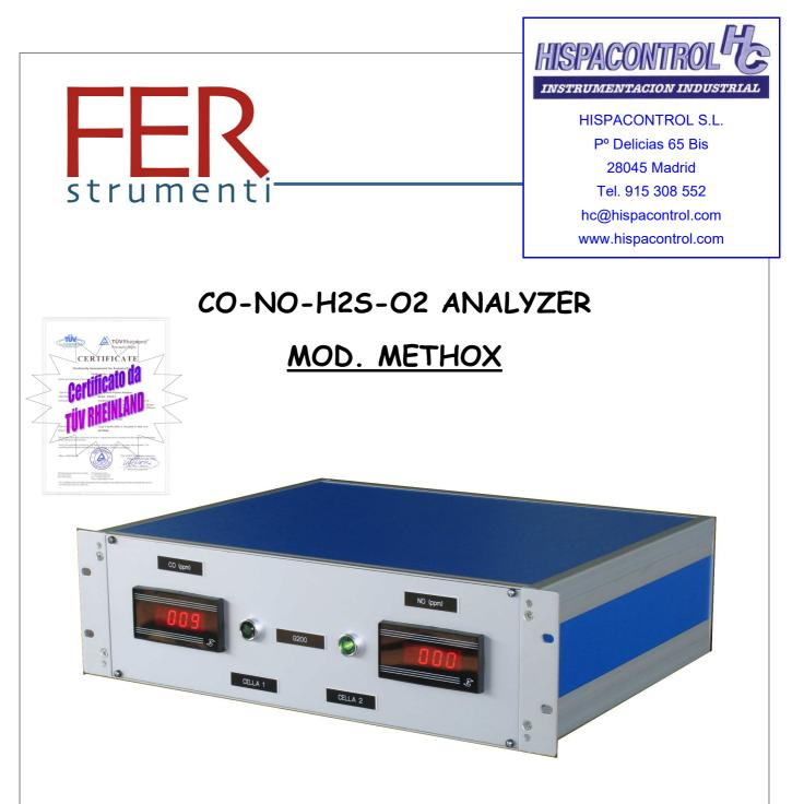
This analyzer technology is based on double cell for CO-NO-H2S and single electrochemical cell for oxygen measurement; it is housed in a rugged 19 "rack. The measurement is displayed on two 7-segment LED display which can also show high or low concentration alarm (independent for each gas). Each alarm is also repeated on a relay contact on the 25-pin connector located on the back of the analyzer.
