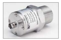
The sensor consists of an anode, electrolyte, and air cathode, together with a diffusion limiting membrane. The rate of diffusion is dependent upon the volume concentration of oxygen in the atmosphere or gas stream. At the cathode, oxygen is reduced to hydroxyl ions, which in turn oxidises the metal anode. The following overall reaction takes place,
