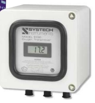
The EC91 Process Oxygen Transmitter will detect levels of oxygen as low as 0.1ppm, up to high percent levels and can be used on most industrial gases and atmospheres. There is no need for routine maintenance of the fuel cell and the instrument can be easily calibrated, using ambient air or standard calibration samples.
