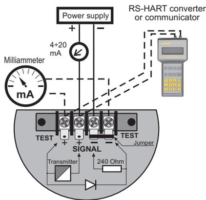
Resistance required for communication (HART) min. 240Ω.
