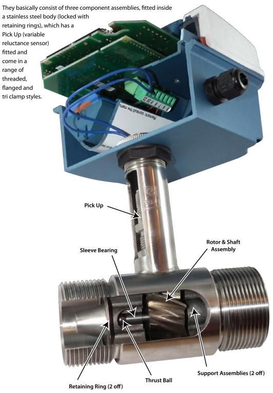
The Rotor and shaft assembly (1 off) which is mounted in sleeve bearings, fitted inside Support assemblies (2 off) is turned by the kinectic energy of the flowing fluid at an angular velocity, which in the linear range of the Flowmeter is proportional to the mean axial velocity of the fluid.
