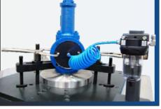
With flange adapters, clamps and bubble jar (API 527)
