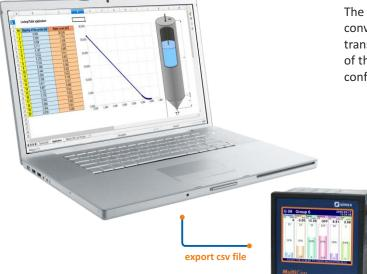
The value of every logical channel of MultiCon recorder may be converted using many various methods: by linear scaling, transfer with compliance to the user characteristics. In the case of the letter, each point of the characteristics required manual configuration, what extended the process significantly.
