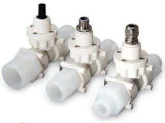
This multi-range radial flow turbine meter uses a low inertia turbine supported on robust sapphire bearings in a chemically resistant housing. 9 flow ranges (0.02 to 160 L/min), a choice of "plug in" fittings and individual traceable calibration make this meter one of the most flexible available. For OEM applications the fittings can be tailored to suit the installation and speed production. Custom leads or connectors are also available for quantity orders.
