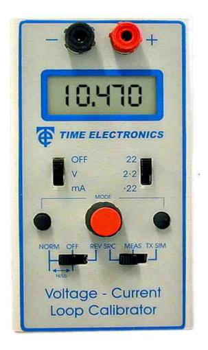
A current, voltage, and process loop calibrator that covers the needs of an R&D lab and process control engineer. Source and measure in three current and voltage ranges plus a transmitter simulator/sink function. It has 4.5 digit (0.005% of span) resolution.
